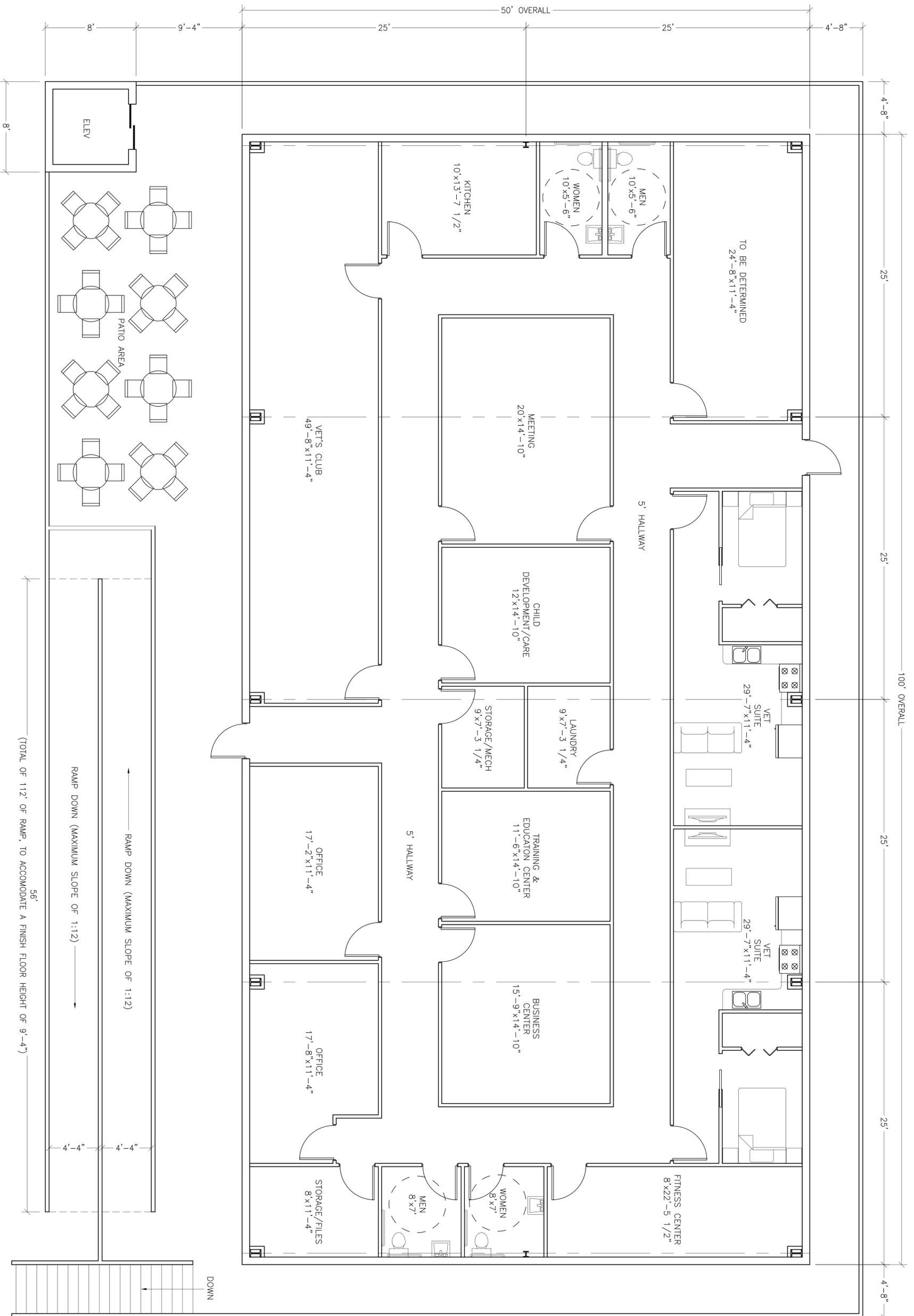
(TOTAL OF 112' OF RAMP, TO ACCOMMODATE A FINISH FLOOR HEIGHT OF 9'-4")
